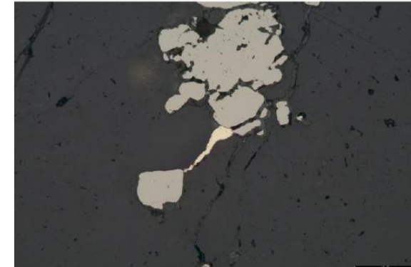
Free milling gold filling fracture in quartz between pyrite.
