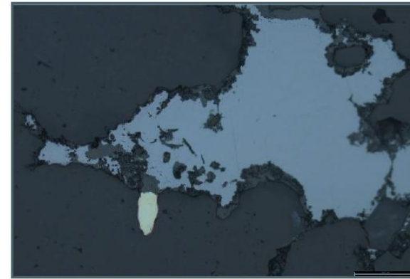
Free milling gold associated with galena.
