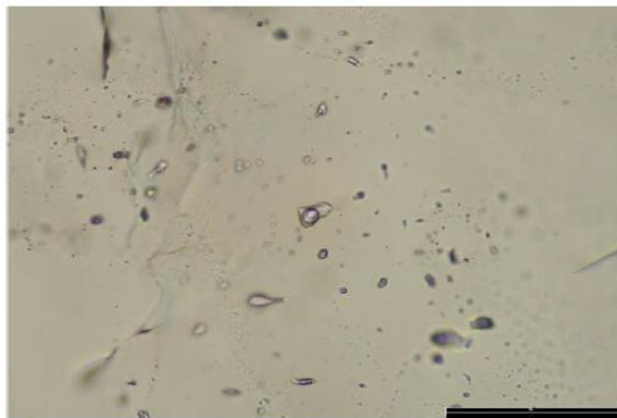
Three-phase fluid inclusion containing aqueous fluid, liquid and gaseous CO 2 .
