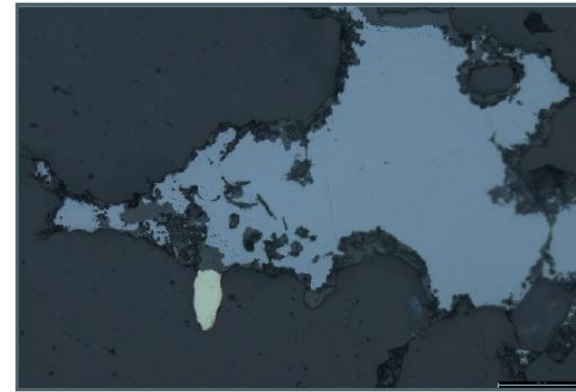
Free milling gold associated with galena.
